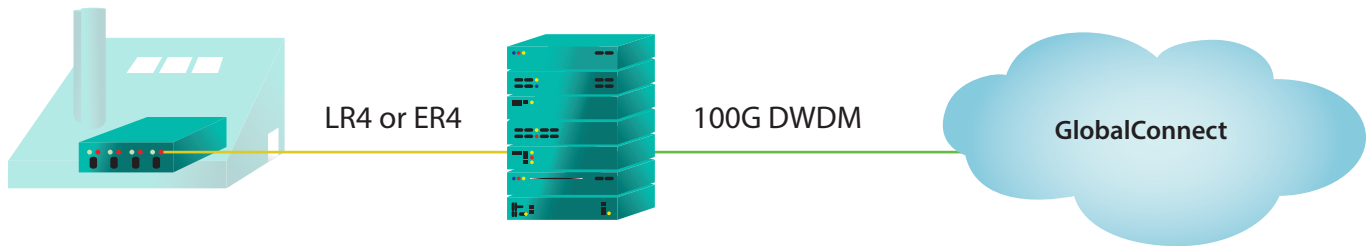
Figure 2: Up to 10 km to GlobalConnect PoP with LR4 and up to 40 km to GlobalConnect PoP with ER4-transceiver.
